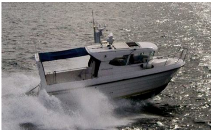
Figure 7. An AUV boat type Viknes designed and developed by the Norwegian University of Science and Technology in conjunction with Marine Robotics (image © Norwegian University of Science and Technology).
