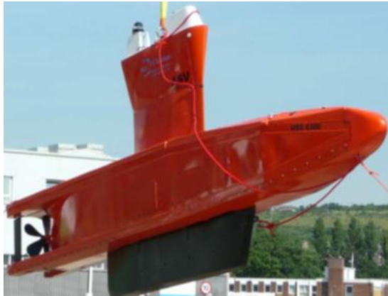
Figure 9. The semi-submersible ASV-6300 designed by C&C Technologies and ASV (image from Wolking, 2011).
