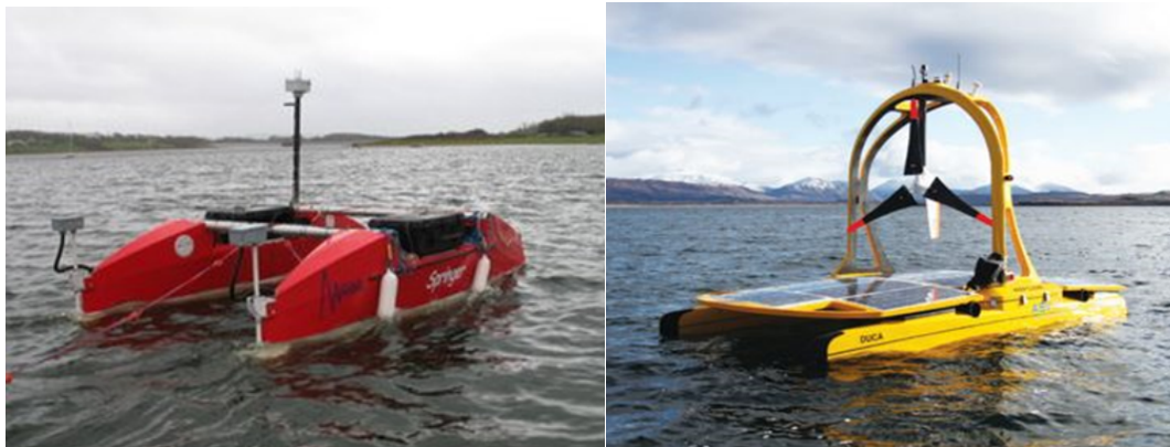
Figure 8. Catamarans: Left picture: Springer, a catamaran based ASV developed by Plymouth University (image © Plymouth University), right picture: ASV C-Enduro, a large scale catamaran based ASV (image © ASV).
